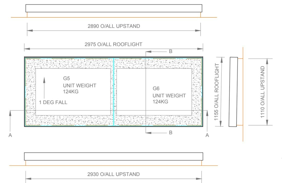
**ALL ROOFLIGHTS DESIGN TO ACCOMMODATE THE FOLLOWING WALK ON LOAD**
